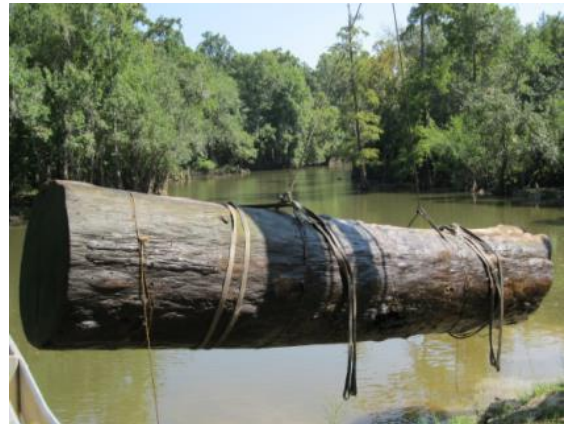
CBF used "sinker cypress" (cypress logs that have been drowned in rivers for years) like the one pictured above as exterior wall finish at the Brock Environmental Center (pictured below).
