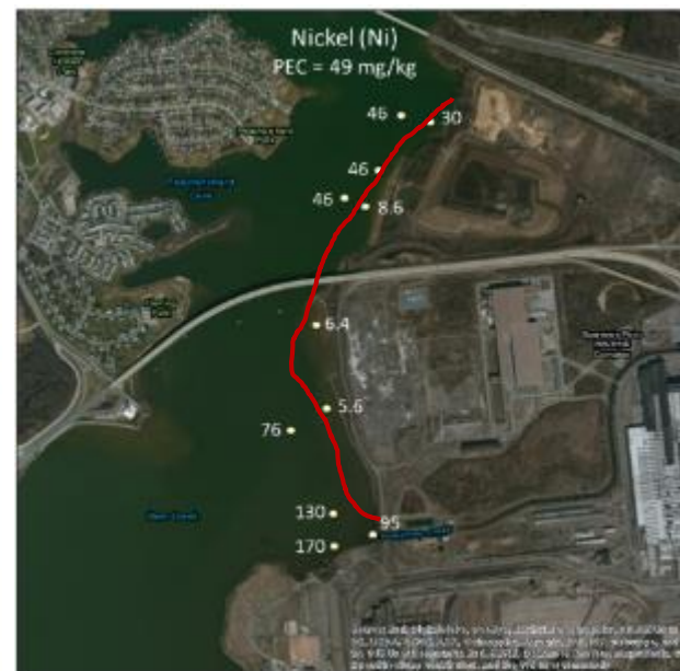
Figure 2. Measured concentrations of zinc (A), chromium (B), copper (C), and nickel (D) at the eleven stations tested for sediment toxicity [values from EA Engineering Technical Memorandum January 14, 2015]. Concentrations in fine sediments from depositional areas (west of red line) often exceeded predicted effect concentration (PEC) levels and revealed a clear north-to-south concentration gradient. Levels in course sandy sediment (east of red line) were generally lower and showed no clear gradient.
