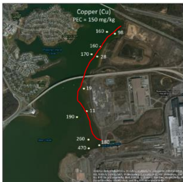
Figure 2. Measured concentrations of zinc (A), chromium (B), copper (C), and nickel (D) at the eleven stations tested for sediment toxicity [values from EA Engineering Technical Memorandum January 14, 2015]. Concentrations in fine sediments from depositional areas (west of red line) often exceeded predicted effect concentration (PEC) levels and revealed a clear north-to-south concentration gradient. Levels in course sandy sediment (east of red line) were generally lower and showed no clear gradient.
